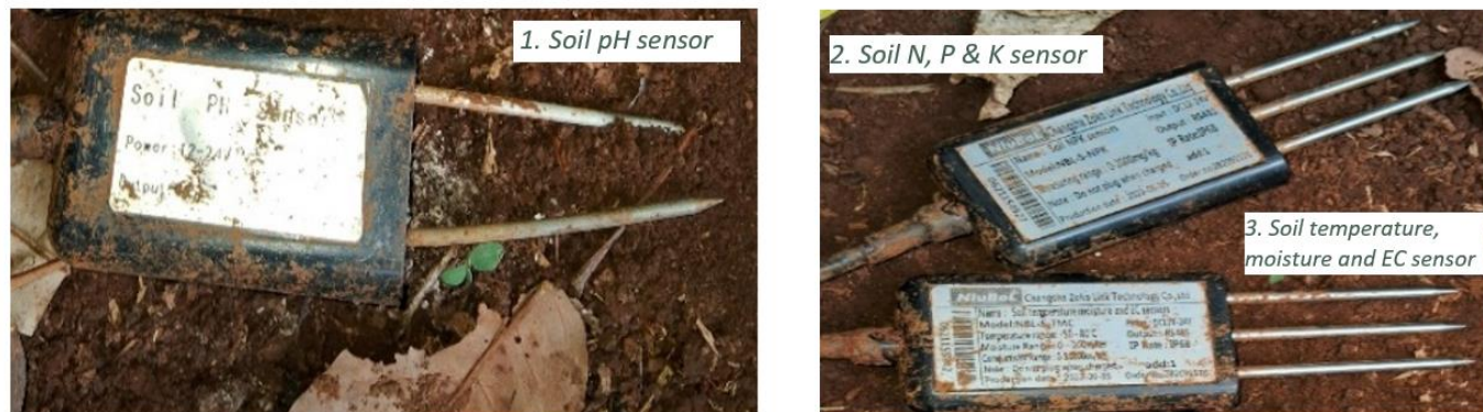
Figure 1 Soil pH, moisture, N, P & K sensors used for study
