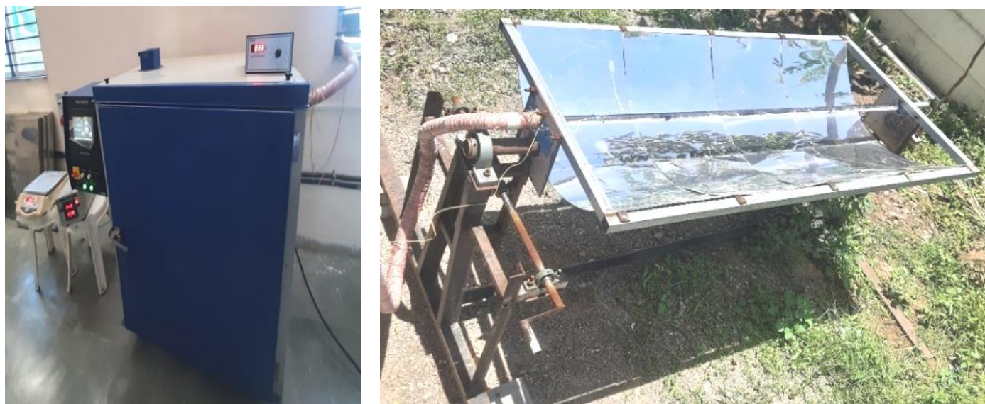
Figure 3 Photograph of assembled solar PTC air heater assisted tray dryer system
