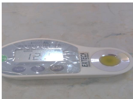
Figure 4. (a) TSS Recording with Digital Refractometer
