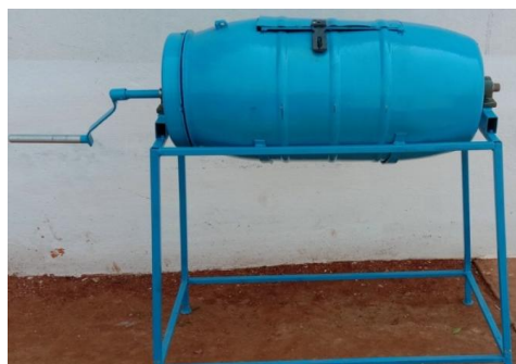
Fabricated in-vessel composter
