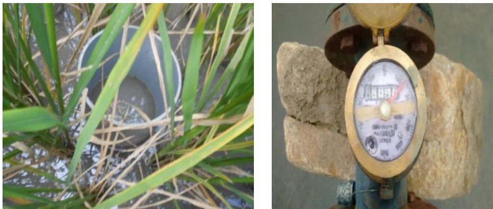
Figure 2 Water measurements in field water tube
