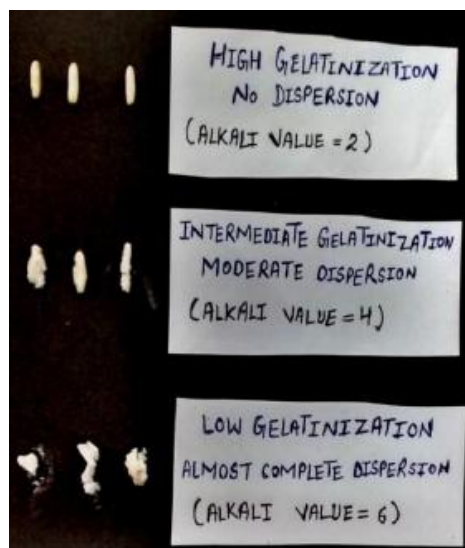
Figure 1 BC 3 F 3 genotypes and parental genotypes were scored based on alkali spread value (ASV) test
