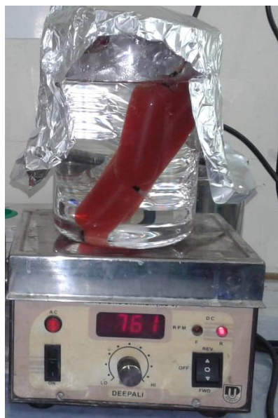
Figure 1 Dialysis of red solution against double distilled water to separate SeNP from oxidized glutathione under magnetic stirring.
