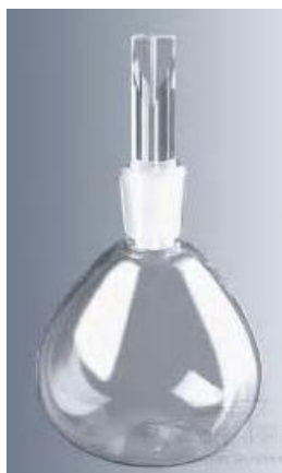
Figure 2 Specific gravity bottle of 25 ml capacity (1, pp 121)
