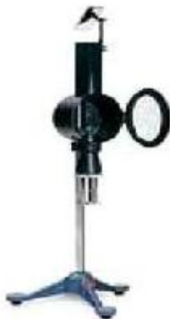
Figure 1 Smoke point (mm) determination lamp as per P 31 IP 57 methodology. (2, pp 146)
