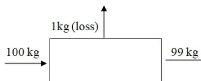
Washer was used for washing the tomatoes. In washer if we feed 100 kg of tomato 99 kg of tomato was obtained as output and there is a loss of 1 kg.
