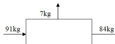
In Pulper-1 coarse particle was used to remove. In pulper on feeding the weighted 91 kg coarse pulp 84 kg thick juice was obtained as output leaving 7 kg as rejected material.
