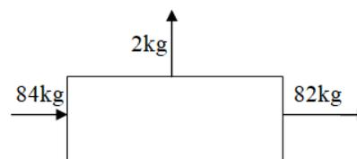
In pulper-2 coarse particles is removed. On feeding 84 kg thicker juice into pulper-2 82 kg thinner juice was obtained as output product leaving 2 kg as rejected material of fine particles.
