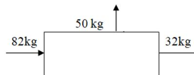
On weighing and feeding the obtained 82 kg output of pulper-2 into evaporator 32 kg of concentrated tomato was obtained as output leaving 50 kg wastage as water.
