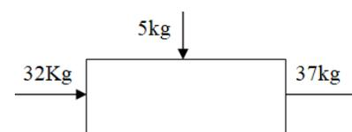
The mixer was used to mix all the ingredients like salt, sugar, preservative etc. which is a weighted quantity of about 5 kg added to the obtained output product of evaporator which was of about 32 kg. Here no loss will occur; here 100% efficiency was achieved.
