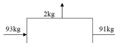
In crusher, crushing of tomatoes is done, in crusher on feeding of 93 kg of tomatoes as input 91 kg of tomato pulp was obtained as output, remaining 2 kg as spill loss.
