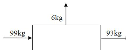
On sorting table, sorting is done to remove foreign matter, in this operation if feed 99 kg of tomato as input 93 kg tomato was obtained as output and 6 kg is lost as impurities.
