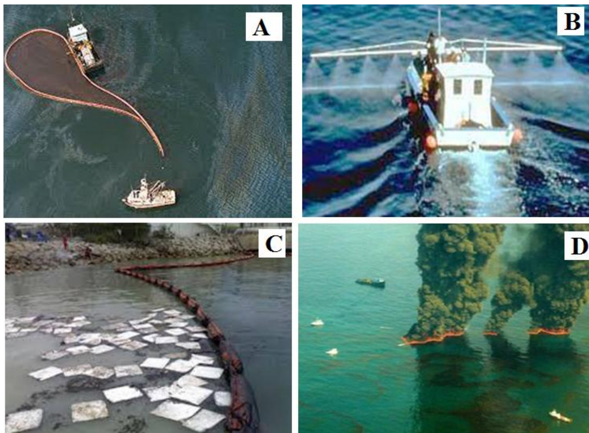
Figure 1 Conventional methods of oil spill cleanup: (A) oil containment with booms; (B) a vessel spraying chemical dispersants; (C) using adsorbents; (D) in-situ burning [10, 25, 34, 35]
