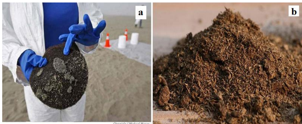
Figure 2 (a) Mat made from a mixture of mushroom & hair, and (b) hyper absorbent peat moss [17]
