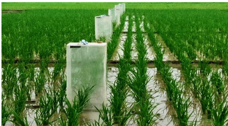
Figure 2 Closed chamber and sampling set up for GHGs (CH 4 and N 2 O) sampling from paddy field, IARI, New Delhi
