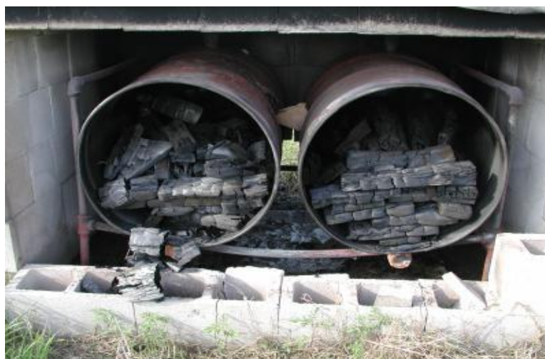
Figure 2 Drum method of biochar production. Source: https://charcoalkiln.wordpress.com/2012/11/10/55-gallon-drum-charcoal-retort/
