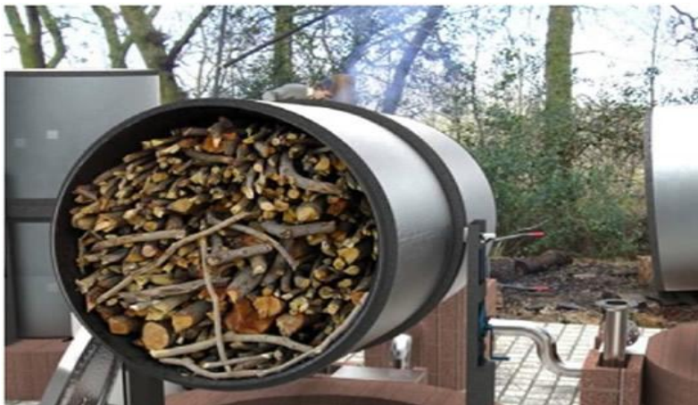
Figure 1 Drum method of biochar production. Source: https://www.pinterest.com/pin/61994932348630789/
