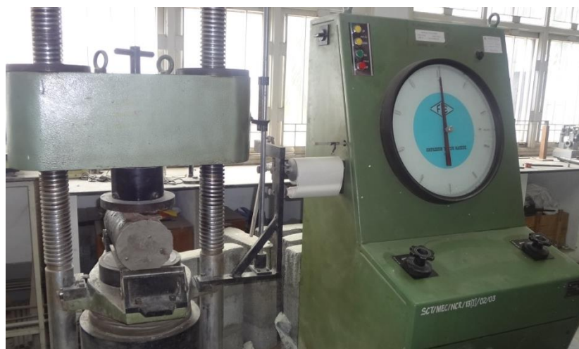
Figure 3 Split Tensile Test on Compression Testing Machine
