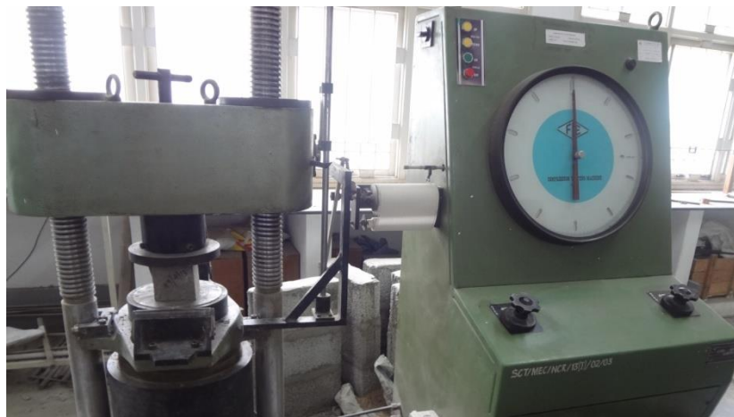
Figure 1 Cube Test on Compression Testing Machine
