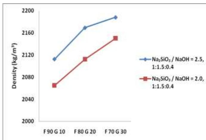
**Figure 6** Density of mortar specimens
