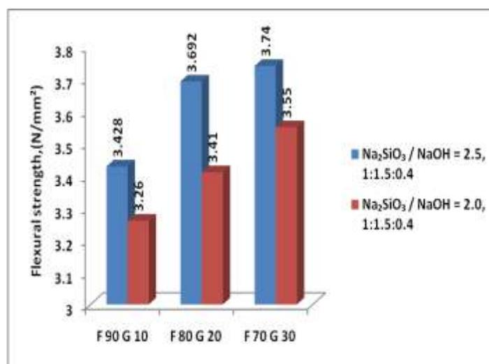
**Figure 8** Effect of  $\text{Na}_2\text{SiO}_3 / \text{NaOH}$  on flexural strength
