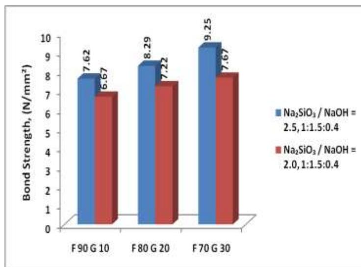
**Figure 9** Effect of Na<sub>2</sub>SiO<sub>3</sub> / NaOH on Bond strength
