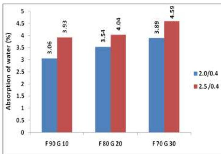
**Figure 10** Water absorption for mortar specimens
