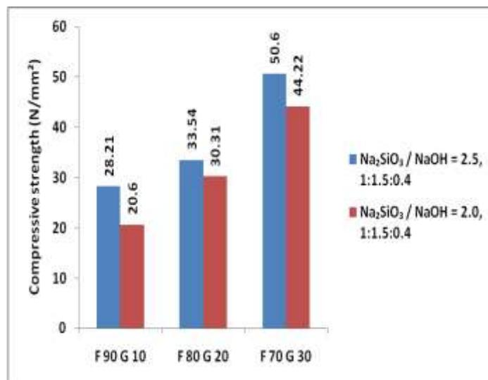
**Figure 7** Effect of  $\text{Na}_2\text{SiO}_3 / \text{NaOH}$  on compressive strength
