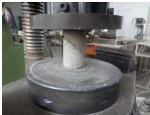
**Figure 3** Slant shear specimen in compression testing machine
