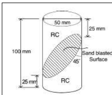
**Figure 2** Diagrammatic representation of slant shear specimen
