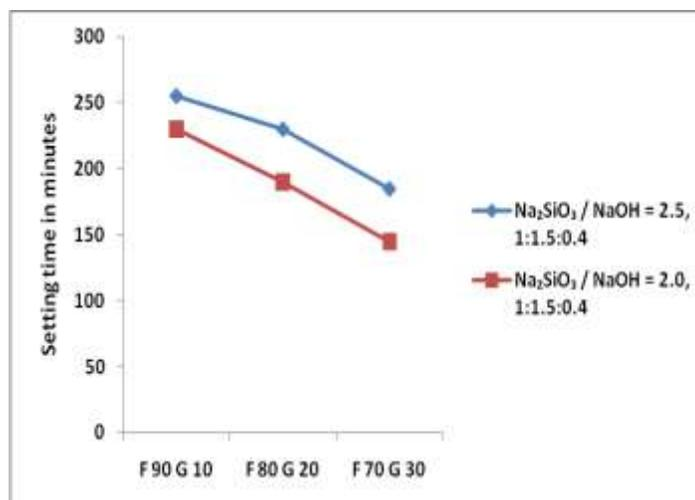
**Figure 4** Effect of Na<sub>2</sub>SiO<sub>3</sub> / NaOH on setting time
