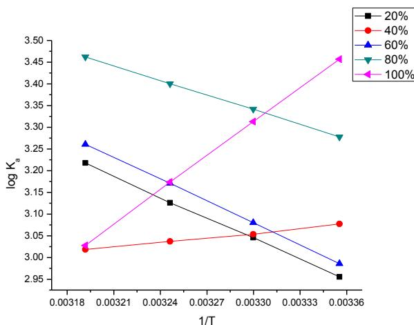
**Figure 3** Relation between  $\log K_A$  versus  $1/T$  for nano  $\text{NiSO}_4$  at different percentage of ethanol-water mixtures
