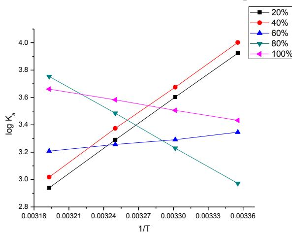
**Figure 4** Relation between  $\log K_A$  versus  $1/T$  for bulk  $\text{NiSO}_4$  at different percentage of ethanol-water mixtures
