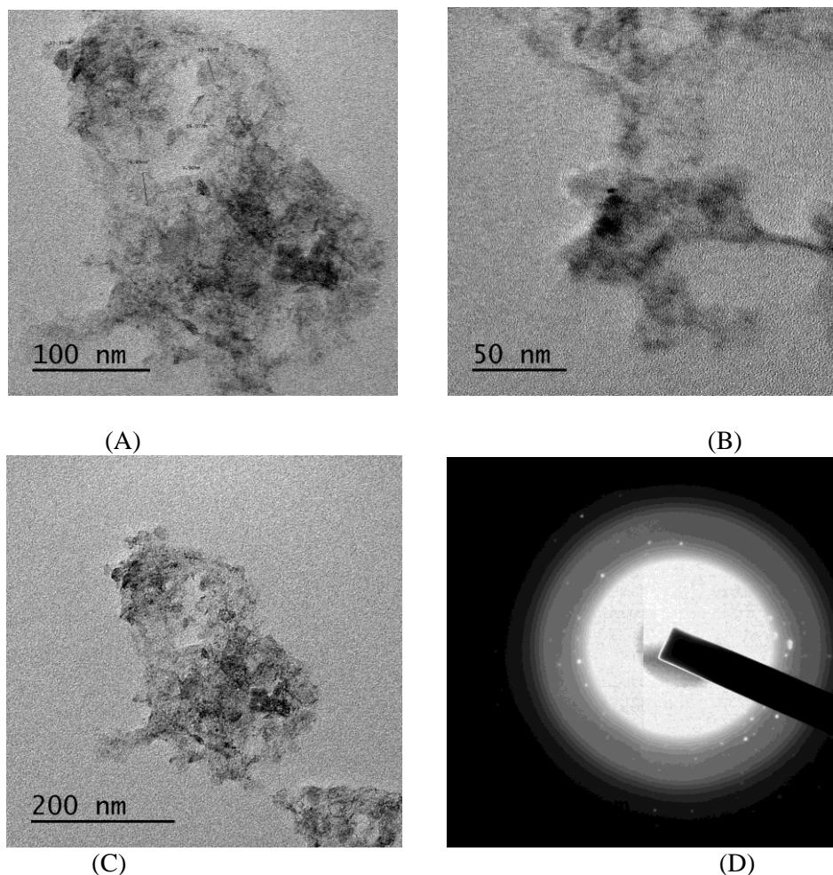
**Figure 2** TEM for nano nickel sulfate
