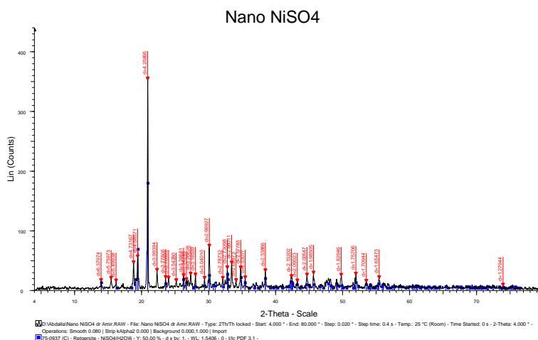
**Figure 1** X-ray diffraction of nano nickel sulfate
