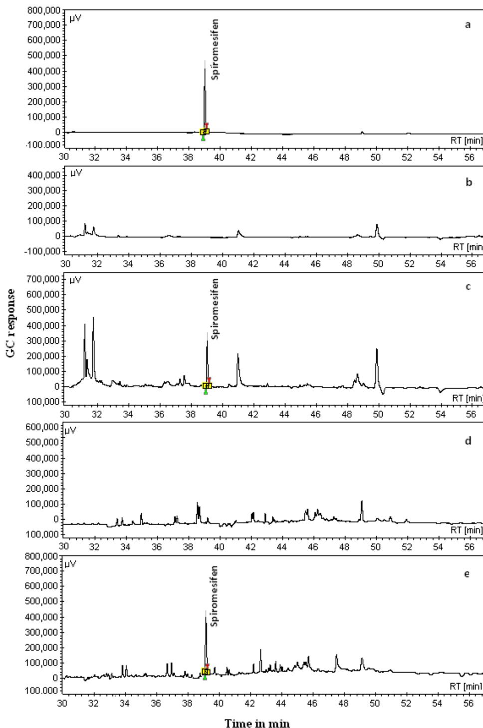
**Figure 2** GC Chromatograms (a) spiromesifen standard at  $0.1 \mu\text{g mL}^{-1}$ , (b) cabbage control, (c) cabbage spiked at  $0.1 \text{ mg kg}^{-1}$ , (d) tomato control, (e) tomato spiked at  $0.1 \text{ mg kg}^{-1}$ .
