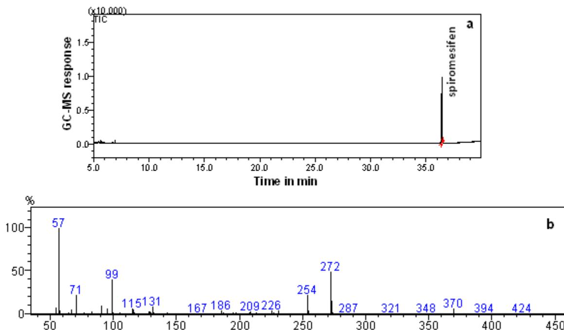
**Figure 3** (a) GC-MS chromatogram of cabbage containing Spiromesifen, (b) mass spectrum of Spiromesifen.
