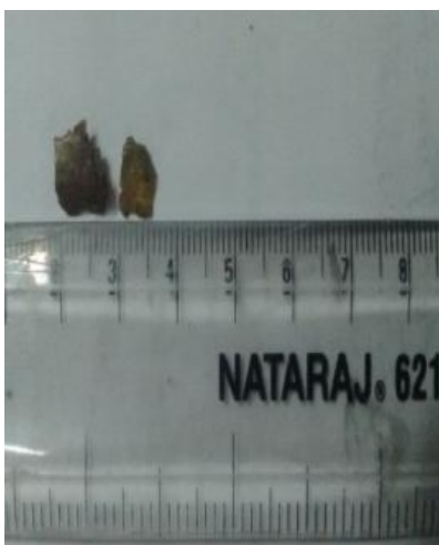
Figure 1 shows Al doped HBA crystal
