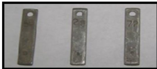
Figure 1 Photograph of mild steel coupons
