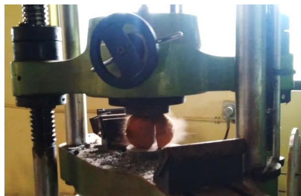
(b) Shell breaking force measurement using Universal Testing Machine
