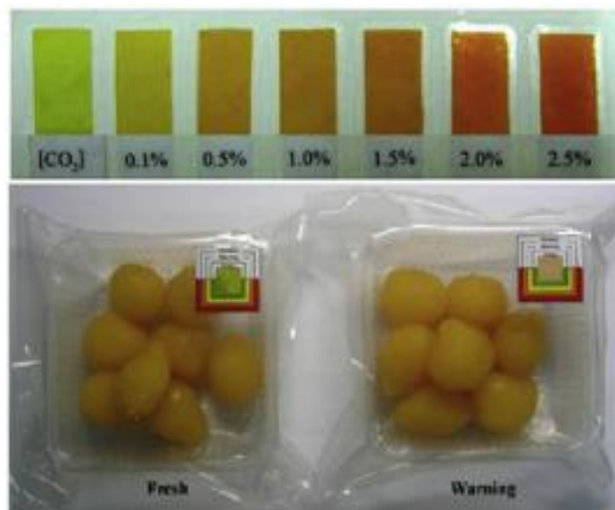
Figure 4 CO 2 gas indicator [34]
