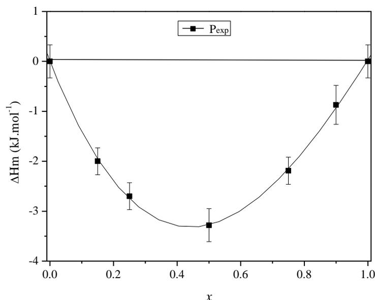
**Figure 1** Variation of enthalpy of mixing as a function of the  $\text{B}_2\text{O}_3$  content of the system  $0.8[x\text{B}_2\text{O}_3-(1-x)\text{SiO}_2]-0.2\text{Na}_2\text{O}$
