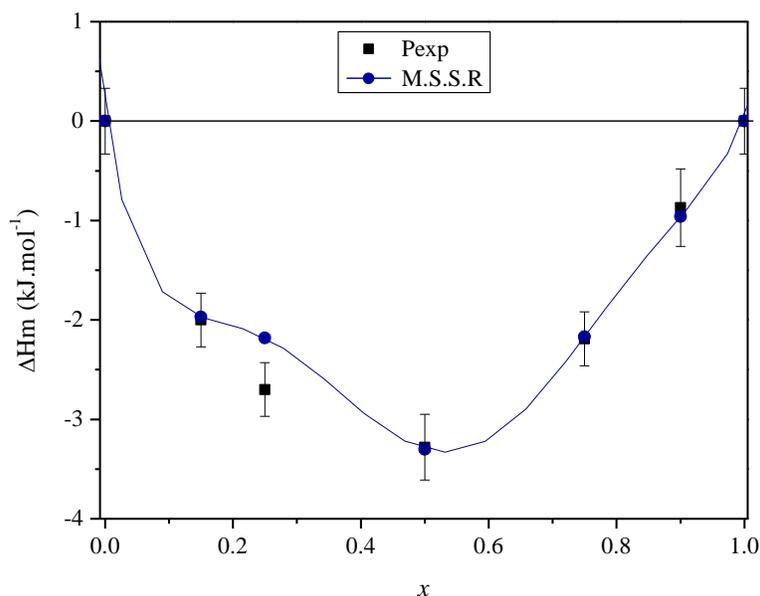
**Figure 2** Experimental values and curve of enthalpy of mixing according to the sub-regular solution model applied to the  $0.8[x\text{B}_2\text{O}_3-(1-x)\text{SiO}_2]-0.2\text{Na}_2\text{O}$  system
