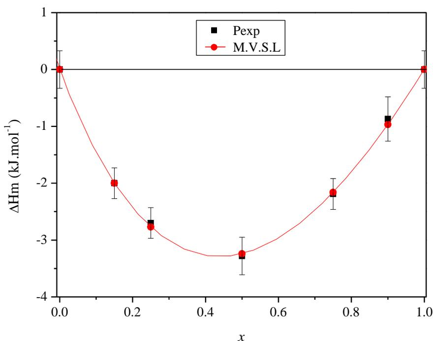
**Figure 3** Comparative study of values of enthalpy of mixing according to the Van Laar model and experimental points
