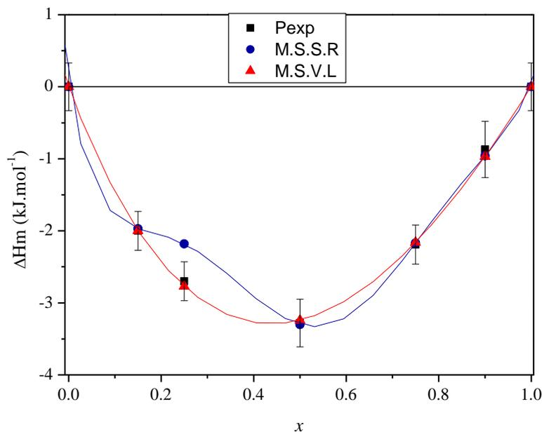
**Figure 4** Comparative study of values of enthalpy of mixing according to the Van Laar and sub-regular solution models
