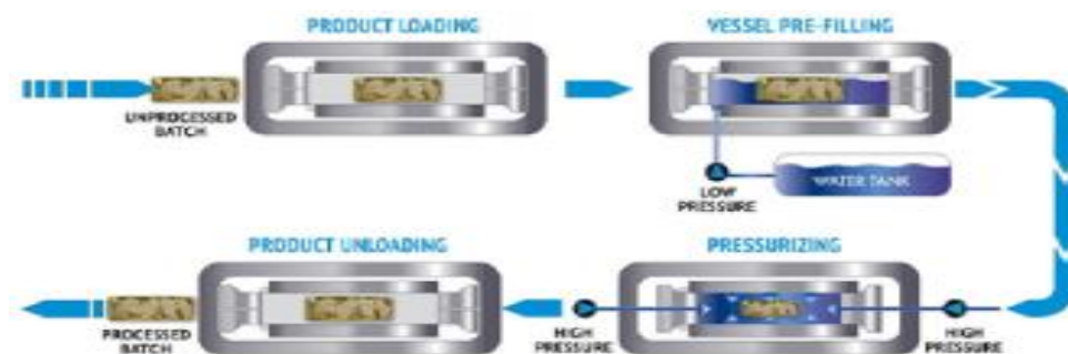
Figure 2 Flow diagram of operation of HPP unit
