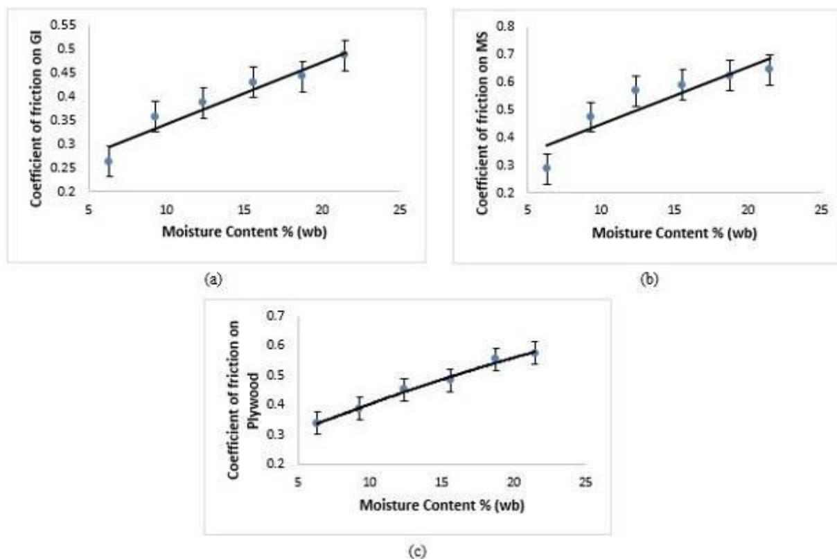
**Figure 8** Effect of moisture content on coefficient of friction of oat on (a) galvanized iron (b) mild steel and (c) plywood surface
