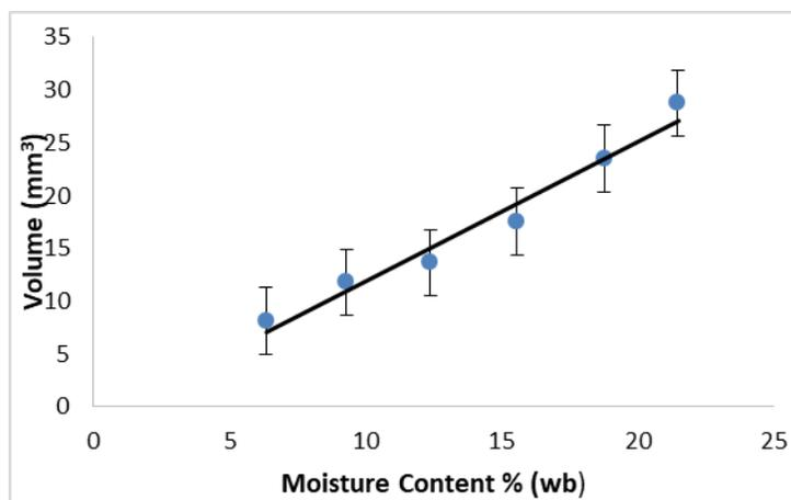
**Figure 2** Effect of moisture content on volume of oat
