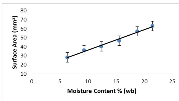
**Figure 3** Effect of moisture content on surface area of oat
