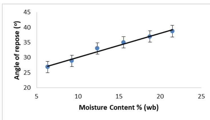
**Figure 7** Effect of moisture content on angle of repose of oat
