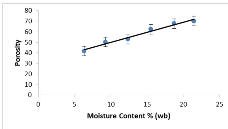
**Figure 6** Effect of moisture content on porosity of oat
