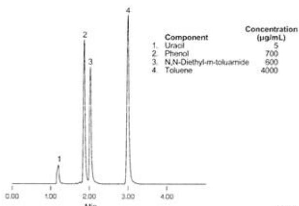
Column: SUPELCOSIL™ LC-18, 25cm x 4.6mm, 5µm particles
