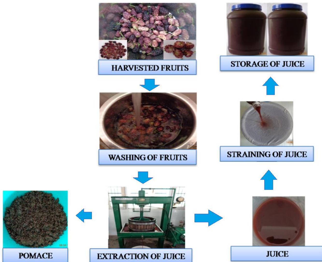
Figure 2 Unit operations for the extraction of juice from mulberry fruit by standardized method
