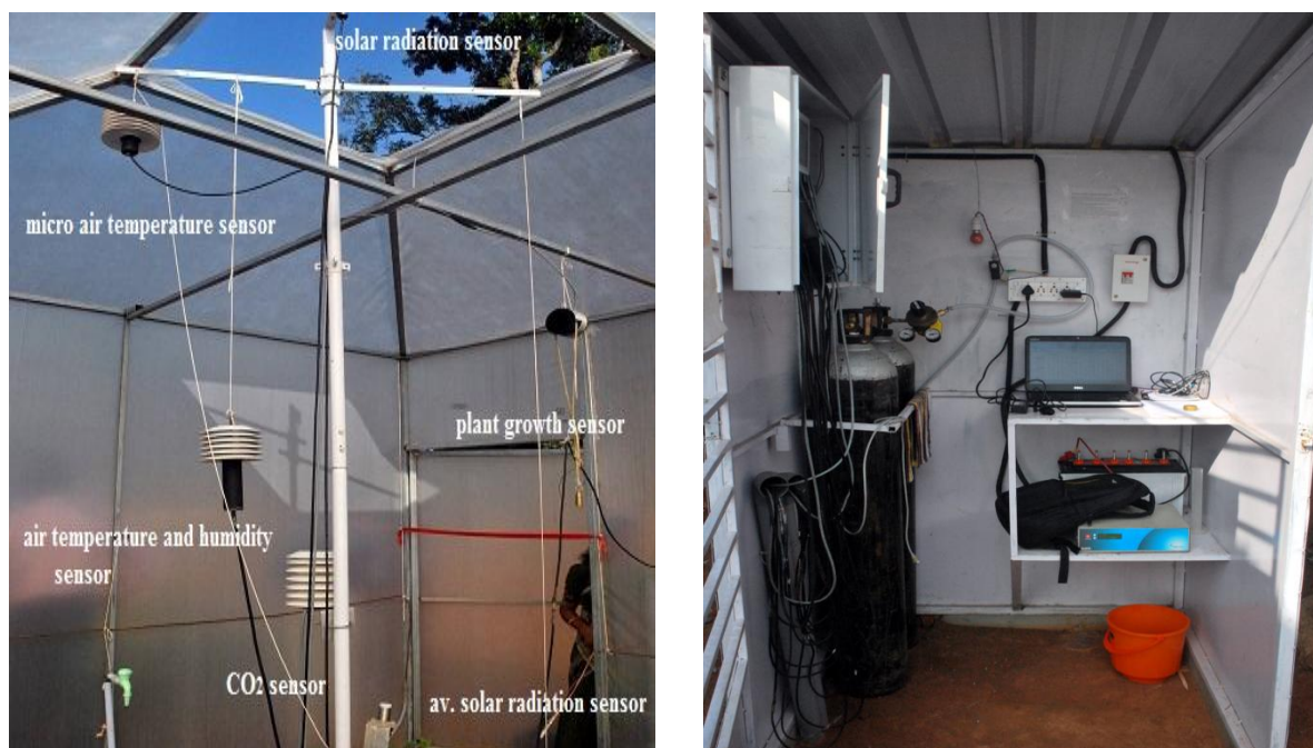
Figure 1 Various sensors and CO 2 cylinders used in open top chamber
