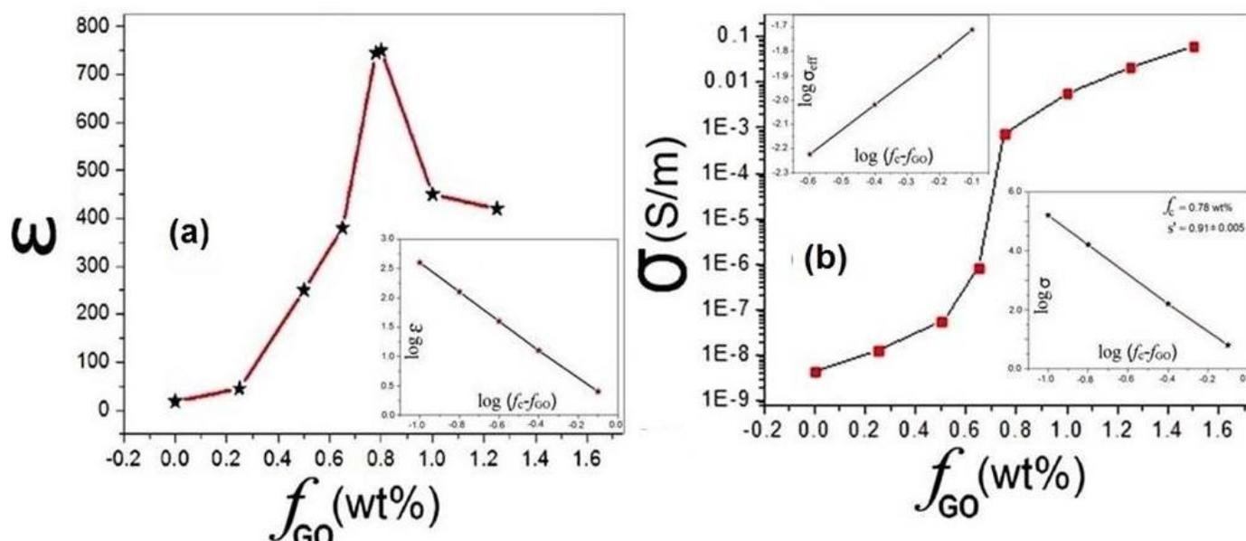
**Figure 2** Dependence of effective dielectric constant  $\epsilon$  (a) and conductivity  $\sigma$  (b) of the PLGA-GO composite on GO concentration  $f_{GO}$ . Inset of (a) shows the best fit of the  $\epsilon$  data with Eq.1 (with  $f_c = 0.78$ ). The inset of (a) and (b) showed the theoretical [12] best fit data of  $\sigma$  data (with  $f_c = 0.78$ ).
