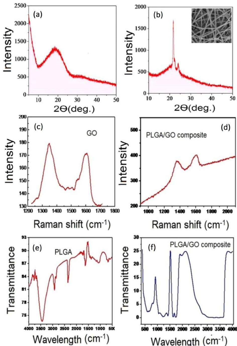
**Figure 1** (a) XRD patterns of pure PLGA and (b) PLGA-GO Composite indicating sharp crystalline peaks. Inset of (b) shows the SEM micrograph of the electrospun PLGA-GO composite fibrous meshes. (c) Raman spectra of GO and (d) PLGA-GO composite meshes. FTIR spectra of (e) PLGA and (f) PLGA-GO composite meshes.
