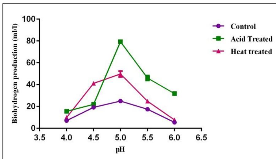
**Figure 2** Cumulative biohydrogen production at different pH with untreated and pretreated effluent
