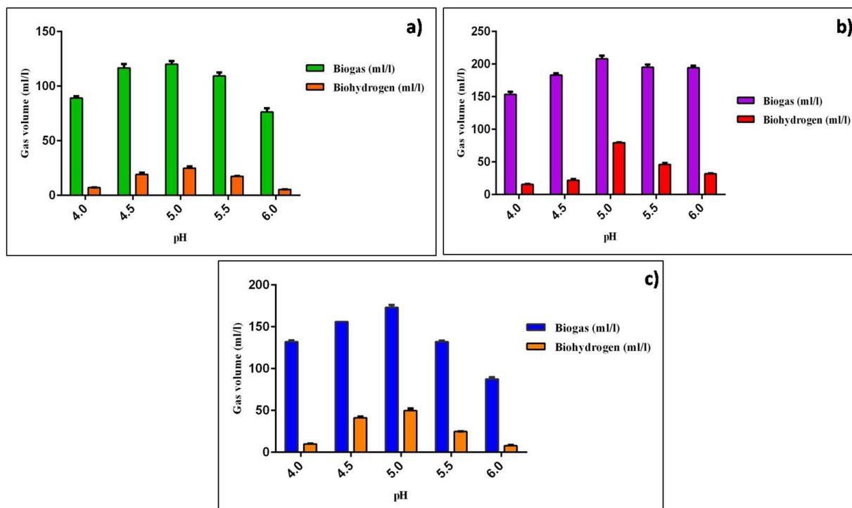
**Figure 1** The cumulative biogas and biohydrogen production at various pH in. (a) USIE, (b) ASIE, (c) HSIE
