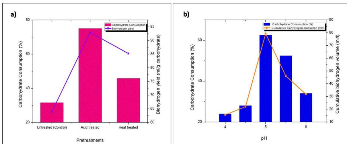
**Figure 3** Carbohydrate consumption rate and (a) biohydrogen yield of USIE, ASIE and HSIE at pH 5 (b) cumulative biohydrogen production at various pH in ASIE
