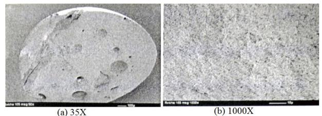
Figure 1 Surface examination of styrene-DVB copolymers cut beads prepared in presence of cyclohexanol diluent
