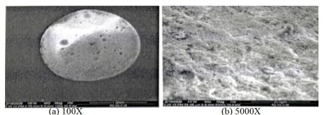
Figure 3 Surface examination of styrene-DVB copolymers cut beads prepared in presence of cyclohexanol-1-butanol mixture in ratio 50-50
