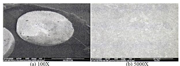
Figure 2 Surface examination of styrene-DVB copolymers cut beads prepared in presence of cyclohexanol-1-butanol mixture in ratio 75-25.
