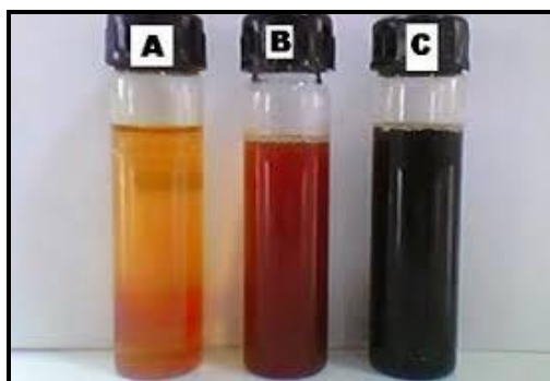
Figure 2 Formation of Iron nanoparticles and its identification by the color change. (A) FeCl 3 solution, (B) plant extract (C) plant extract with FeCl 3 solution.
