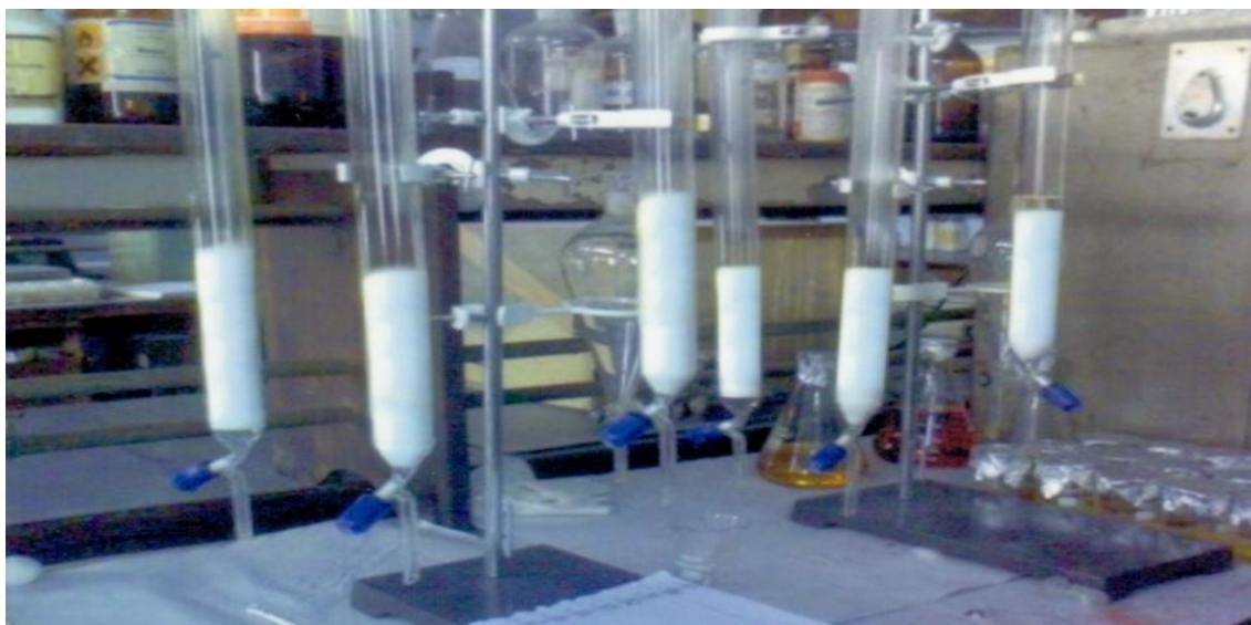
Figure 2 Filling of column chromatography
