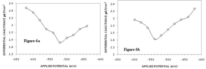
**Figure 6** Plot of Applied potential vs differential capacitance for mild steel in 1.0 M HCl (a) and 1.0 M HCl containing 300 ppm of 2 PPT (b)
