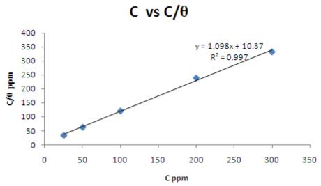
Figure 7 Langmuir's Isotherm for adsorption of inhibitor molecules onto mild steel surface in 1.0 M HCl solution.
