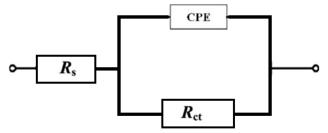
Figure 4 Equivalent circuit for mild steel corrosion in 1.0 M HCl solution.
