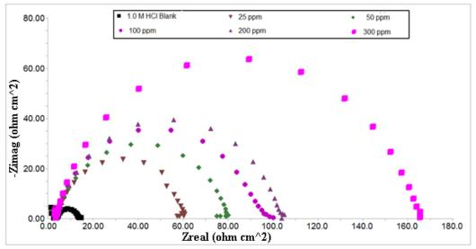
Figure 3 Nyquist plots for mild steel in 1.0 M HCl in the absence and presence of 2 PPT
