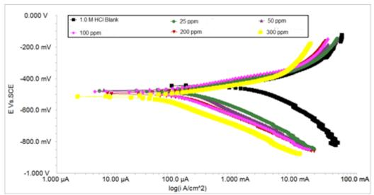
Figure 5 Tafel plots for mild steel in 1.0 M HCl in the absence and presence of 2 PPT
