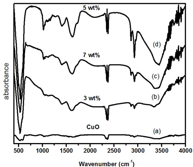
Figure. 2 FT-IR spectrum of undoped (a) CuO and (b) 3 (c) 7 and (d) 5 wt% of Indium doped with CuO.
