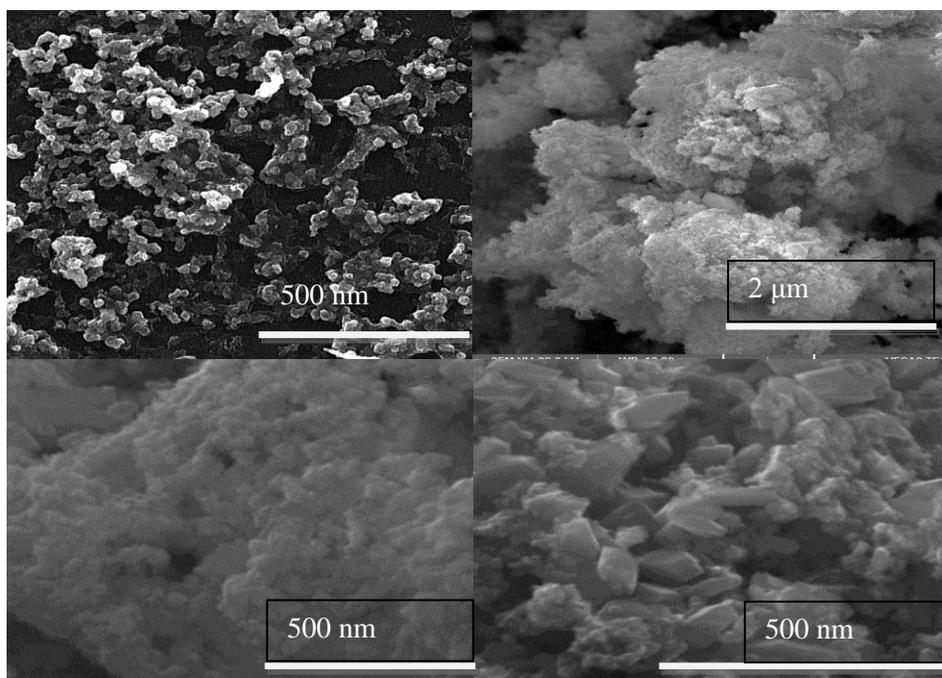
Figure 4. SEM images of (a) undoped CuO and b, c and d of 5 wt% Indium doped with CuO
