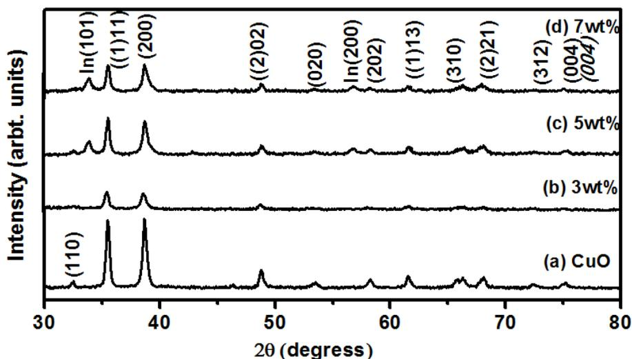
Fig.1 XRD patterns of (a) undoped CuO and (b) 3 (c) 5 and (d) 7 wt% of Indium chloride doped with CuO
