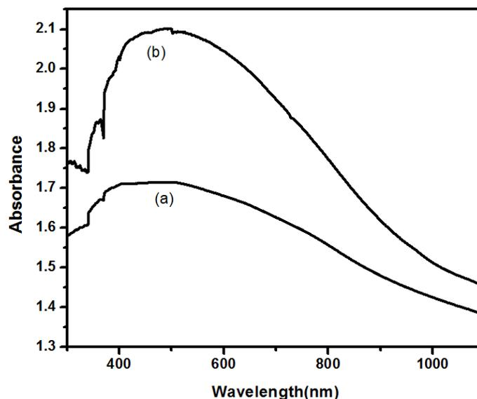
Fig 3. UV-Visible spectra of a) CuO and b) In doped CuO nanoparticles.
