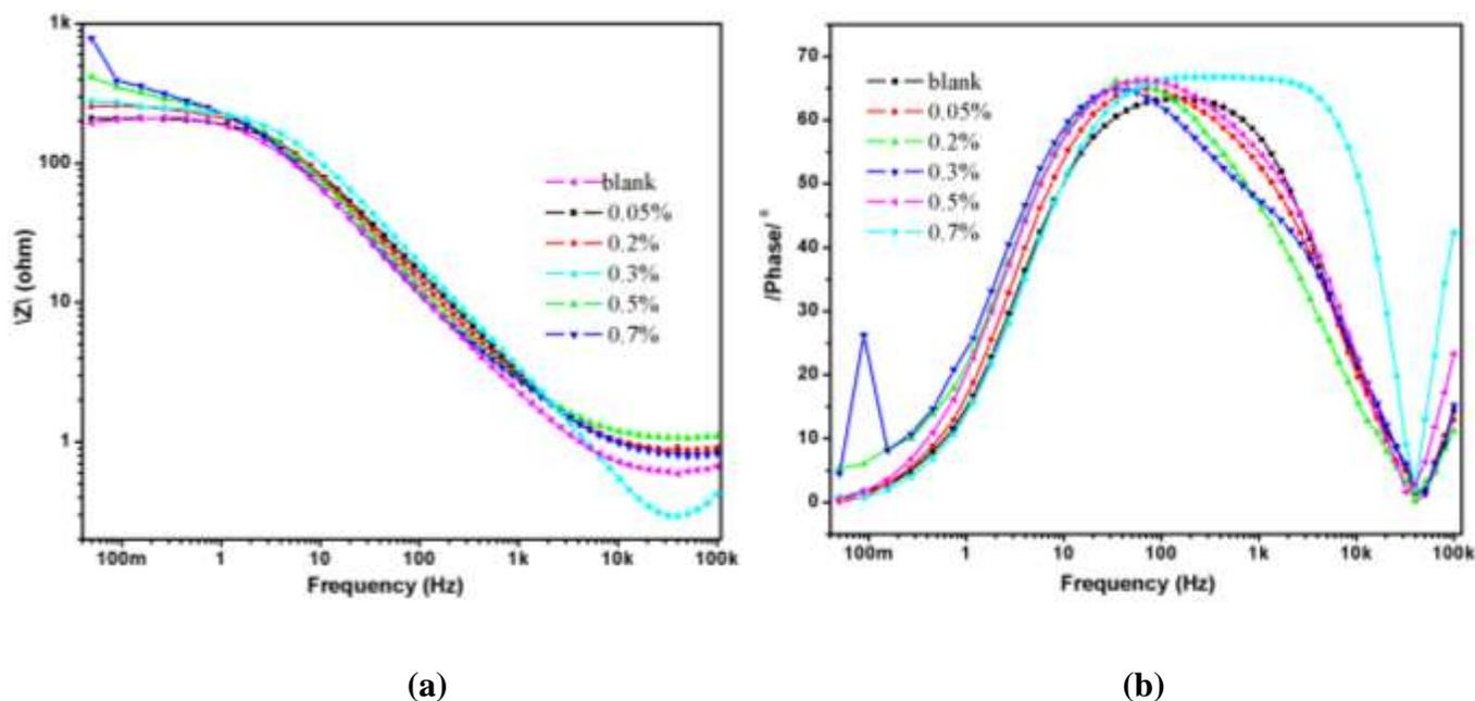
**Figure 2** Bode plots for mild steel in 1M HCl in the presence and absence of Ai extract
