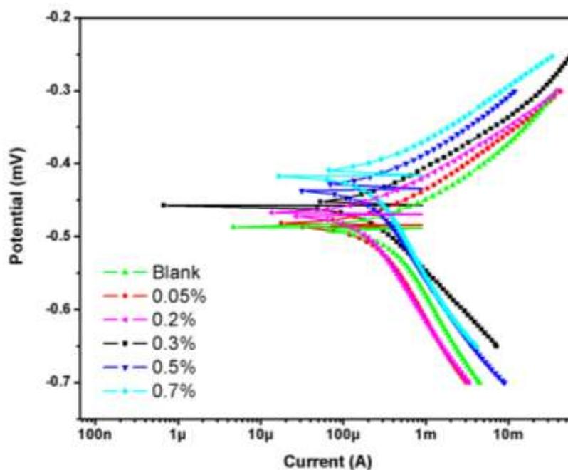
**Figure 1** Potentiodynamic polarization curves for mild steel in 1M HCl in the absence and presence of different concentrations of Ai extract
