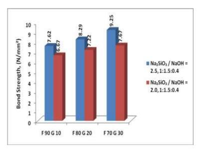
Figure 9 Effect of Na<sub>2</sub>SiO<sub>3</sub> / NaOH on Bond strength
