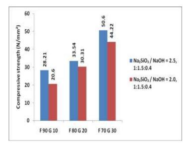
Figure 7 Effect of Na<sub>2</sub>SiO<sub>3</sub> / NaOH on compressive strength
