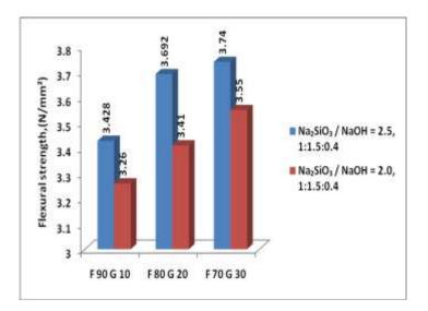
Figure 8 Effect of Na<sub>2</sub>SiO<sub>3</sub> / NaOH on flexural strength
