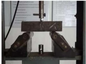
Figure 1Testing of prism
