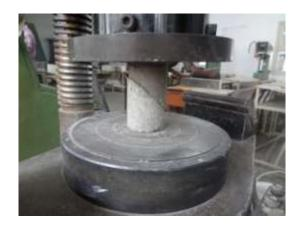
Figure 3 Slant shear specimen in compression testing machine
