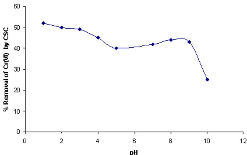
**Fig.2** Effect of pH on Adsorption of Cr (VI) of Concentration 10mg /L-Time: 3hrs: Carbon Dose 100mg/100mL; pH: 5.0-9.0
