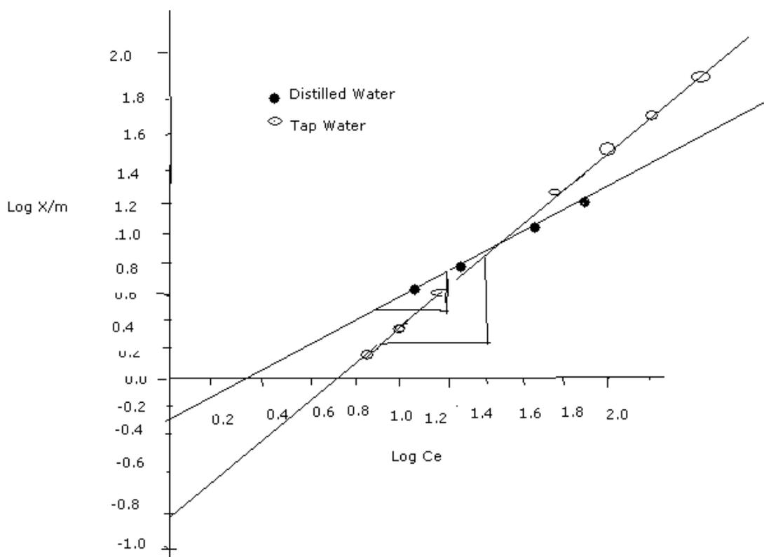
**Fig.6** Freundlich Adsorption Isotherm for the Adsorption of Cr (VI); Time: 10Hrs: pH: 1
