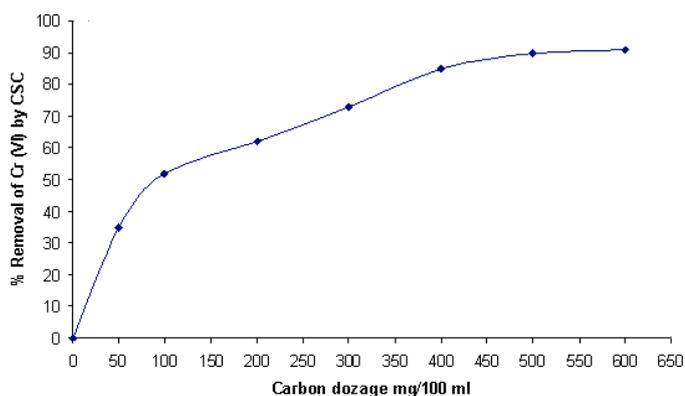
**Fig. 3** Effect of Carbon Dosage pH 1
