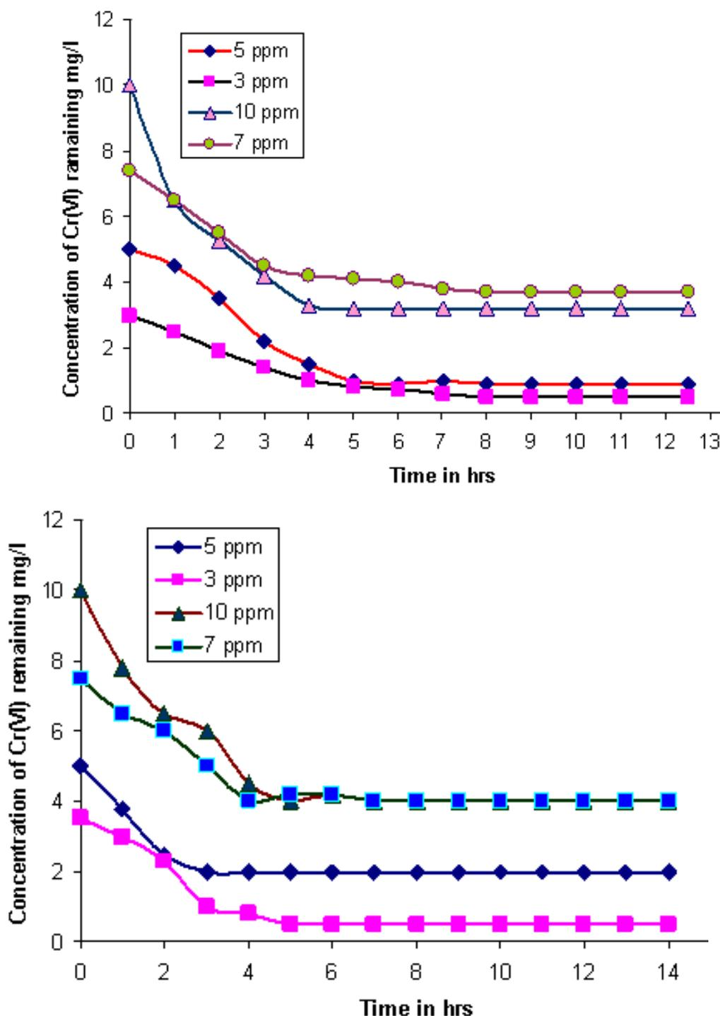
Fig 7. First Order Kinetic Fit for the Adsorption of Cr (V) on CSC
