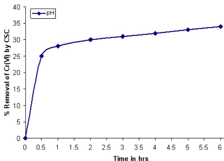
**Fig.1** Effect of Time for the Removal of Cr (VI) of Concentration 10mg/L-Carbon Dose 100mg/100mL; pH: 5.0
