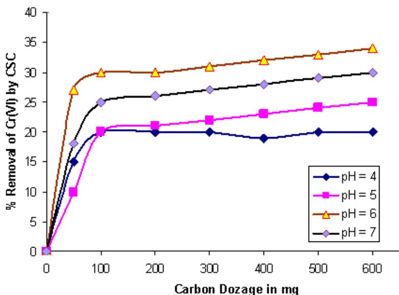
**Fig. 5** Effect of Carbon Dosage on Adsorption of Cr (VI) of Concentration 10mg/L- Time 3Hrs; pH 4 to 7
