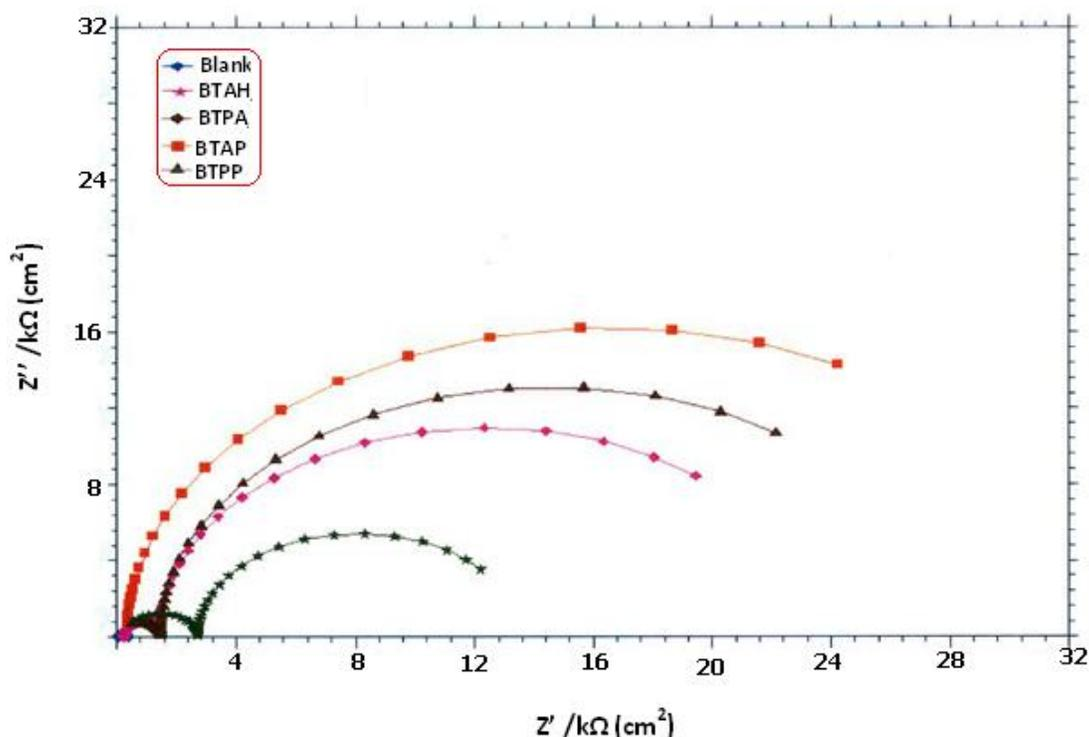
**Figure 4** Nyquist diagram of Al-brass in solution containing optimum concentrations of HMBT, natural sea water
