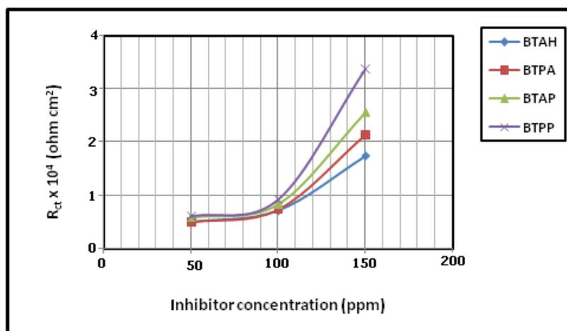
**Figure 5** Variation of  $R_{ct}$  values with different concentration of BTAH, BTPA, BTAP and BTPP in natural sea water
