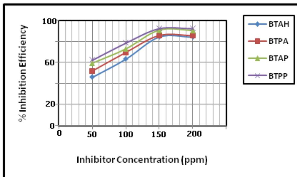
**Figure 2** Variation of inhibition efficiency with different concentration of BTAH, BTPA, BTAP and BTTP in natural sea water
