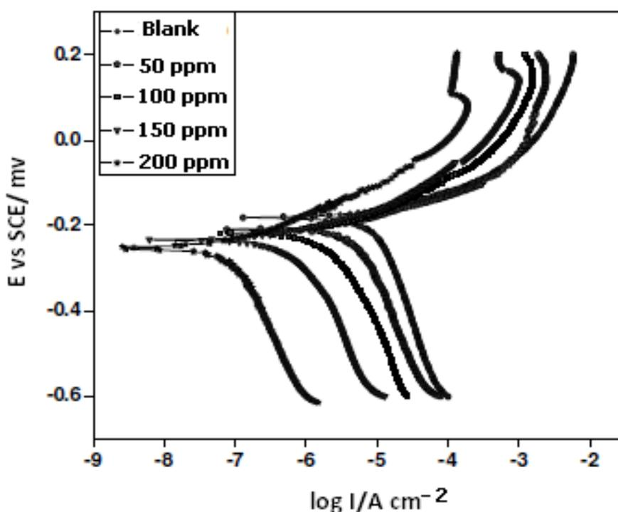
**Figure 3** Polarization curves of Al-brass in natural sea water containing optimum concentrations of BTAH, BTPA, BTAP and BTTP
