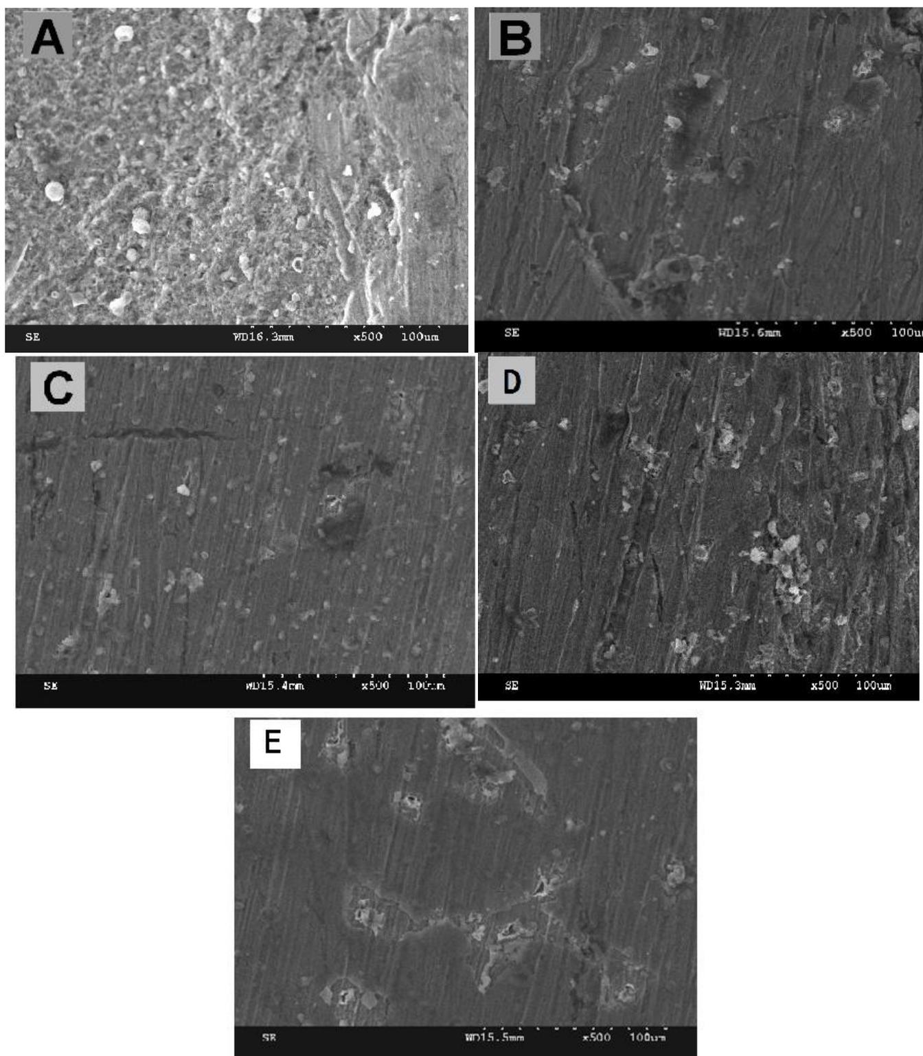
**Figure 7** SEM micrographs of Al-brass immersed in natural sea water with BTA derivatives (A) Blank, (B) BTAH, (C) BTPA, (D) BTAP and (E) BTTP
