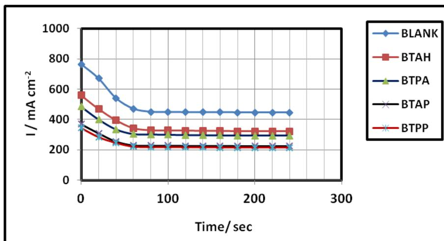
**Figure 6** Potentiostatic current transient curves of Al-brass in natural sea water containing optimum concentration of BTAH, BTPA, BTAP and BTPP
