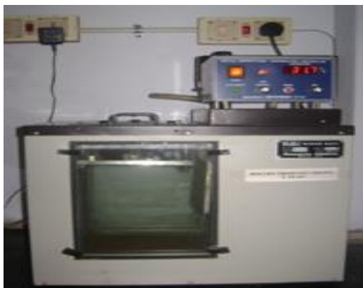
Figure 3 Photograph of thermostat (Raaga Lit pump type digital)
