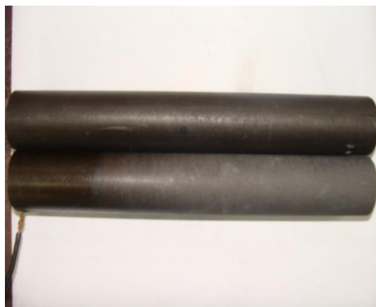
Figure 2 Corrosion of graphite electrode
